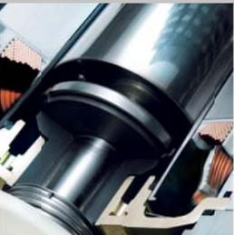
The smaller rotor is designed for speeds ranging beyond 4,000 RPM. This has reduced the size and weight of the motor housing, permitting easier handling with the same power.
